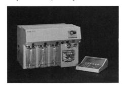
row-bore (0.21-cm) columns. A tested column and documentation come with the BAS-200 PTH. All phenylthiohydantoin derivatives are resolved in 18 min, with a
