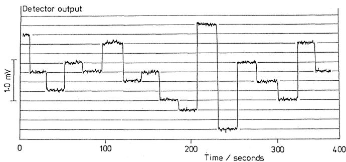
**Fig. 1.** Output of SQUID magnetometer showing small integral numbers of flux quanta jumping in and out of a ring of  $Y_{1.2}Ba_{0.8}CuO_4$ . Step heights provide proof of existence of pairs. [Courtesy C. Gough (7), reprinted with permission of *Nature*, copyright 1987, Macmillan Journals Ltd.]
