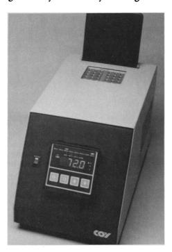
ing and cooling stages between 0° and 105°C. The model 50 TEMPCYCLER can store eight temperature profiles, each consisting of as many as six independent ramp and soak intervals. Thermoelectric modules cool the samples faster than cooling by water and more cheaply than cooling by compressed gas. Samples may be frozen at the end, if desired. Coy Laboratory Products. Circle 512.
