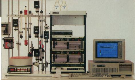
FPLC System takes you through your entire separation strategy – increasing the efficiency of your methods development and optimizing your final purification scheme – all with the intelligent system control and data handling capabilities of FPLCmanager.
