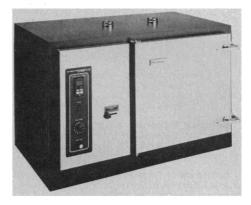
kg/m<sup>2</sup>), and the front door releases at pressures more than 50 lb/ft<sup>2</sup> (244 kg/m<sup>2</sup>). The oven conforms to the National Fire Protection Association 86 safety specification. The oven's chamber is stainless steel and has a 4ft<sup>3</sup> (0.11-m<sup>3</sup>) capacity. The digital alarm is backed up by a mechanical alarm, and there is also a temperature deviation alarm. Precision Scientific. Circle 529.
