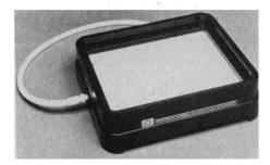
rubber mask, and a gel on a 19 by 24 cm perforated stainless steel screen over the vacuum chamber. When the top is in place, the resulting chamber can be filled with transfer buffer. Nucleic acids are transferred to the membrane as buffer is drawn down through the gel and the membrane by the vacuum. Hoefer Scientific Instruments. Circle 528.
