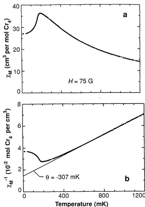
**Fig. 4.** The dc molar magnetic susceptibility (a) and its inverse (b) versus temperature for  $[\text{Cr}_4\text{S}(\text{O}_2\text{CCH}_3)_8(\text{H}_2\text{O})_4](\text{BF}_4)_2 \cdot \text{H}_2\text{O}$  between 13 mK and 1.2 K. The data have been normalized to the data in Fig. 2 above 1 K.
