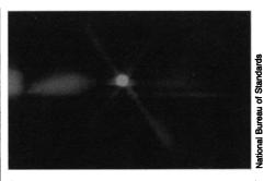
**Six laser beams meet,** creating a region of "optical molasses" that holds atoms of sodium gas.
