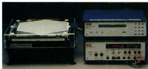
THE PULSAPHOR SYSTEM INCLUDES AN ELECTROPHORESIS UNIT, POWER SUPPLY AND CONTROL UNIT.
