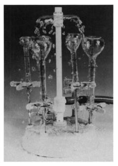
with a continuous water stream containing air bubbles. The flasks are held in place by clips. A variable sprinkler adjust valve allows the water to spread over the flasks. The WASHMAN can rinse six flasks of different sizes. Rael Laboratories. Circle 571.
