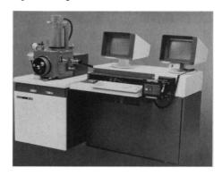
fixed, dehydrated, or subjected to critical-point drying. Because the Wet-SEM can operate with high electron beam energies, an optional energy-dispersive x-ray detector enables it to provide elemental analysis. Magnifications from  $\times 10$  to  $\times 150,000$  are possible. Samples can be as large as 15 cm in diameter. \$72,500. International Scientific Instruments, Circle 538.
