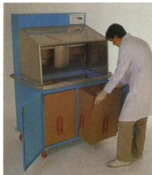
Removing optional burn box with polyvinyl liner.
