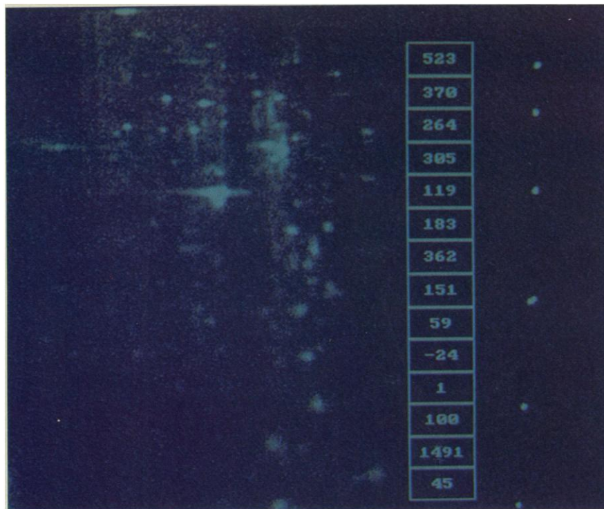
AMBIS screen image of 2-D gel analysis of ^{35}\text{S} -labeled whole cell proteins from murine Swiss 3T3 fibroblasts. Number in second box from bottom of screen, 1491, indicates quantitation of radioactivity in calmodulin. Courtesy of Herbert L. Cooper, National Cancer Institute.
