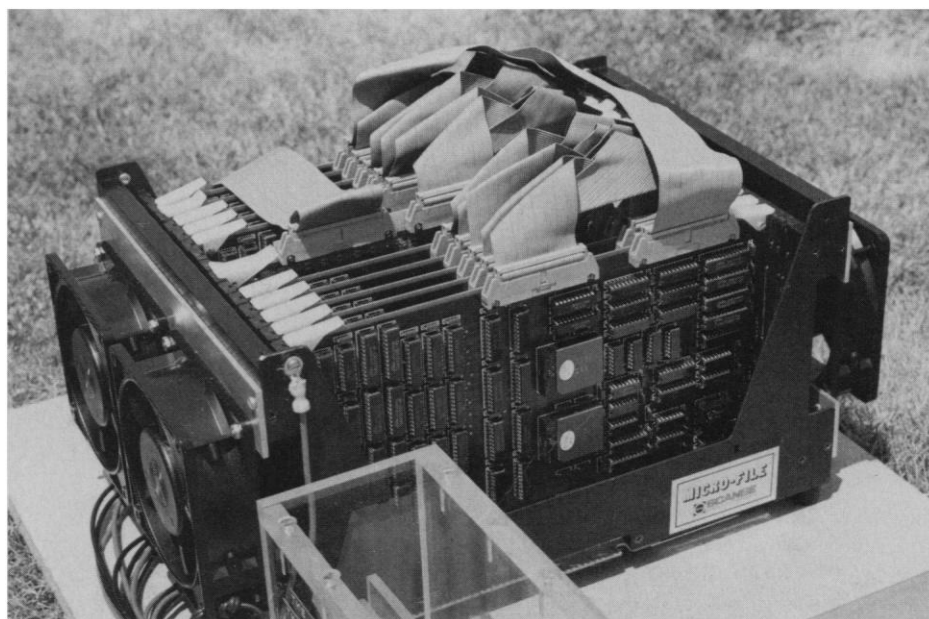
The new and the old orreries. The mechanical calculation of the positions of the planets began in the 17th century with the original form of the orrery (right), named after the Earl of Orrery for whom it was first made. The Digital Orrery (above), a one of a kind parallel computer, is less stylish but much faster. Designed solely for simulating the motions of the solar system, it runs at one-third the speed of a Cray 1 supercomputer.
