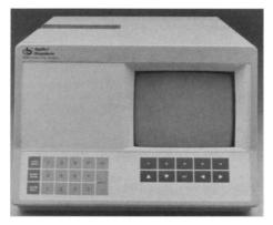
monitor absorbance at different wavelengths and ranges. The user can capture complete spectral scans anytime during operation through time-based programming or the built-in peak-detection software. Wavelengths may be changed instantaneously at any time. Applied Biosystems, Ramsey Analytical Division. Circle 565.
