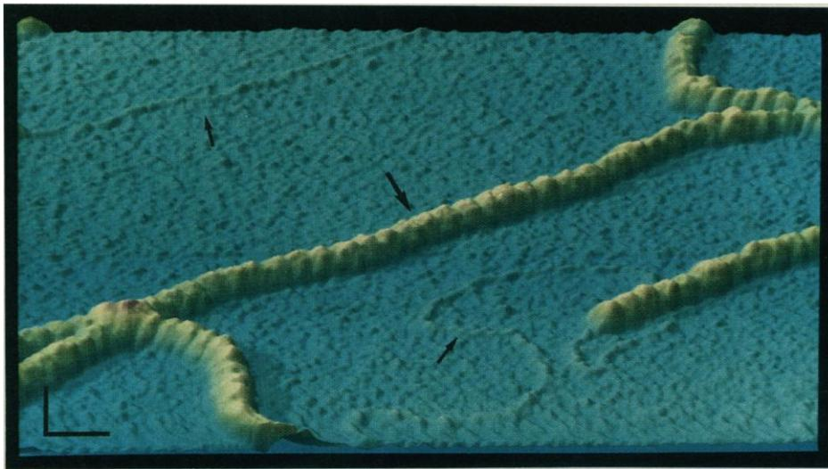
**Fig. 2.** Processed STM image with simulated shading of freeze-dried recA-DNA complexes coated with a Pt-Ir-C film. The area corresponds to 236 nm by 192 nm. Large arrows point to recA-DNA complex; small arrows point to free DNA. The bars denote a distance of 20 nm in each direction.
