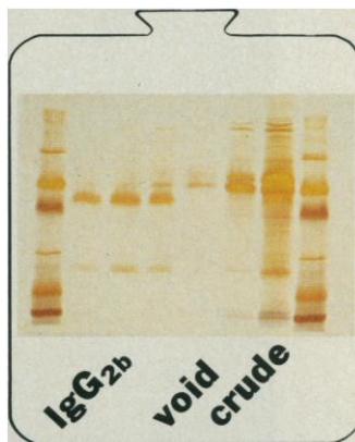
Monitoring IgG 2b purification with SDS-PAGE on PhastGel Gradient 10-15 with sensitive silver staining. From sample to result: 90 min.
