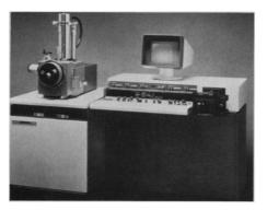
diameter. The microscope operates at accelerating voltages from 1 to 30 kV, allowing it to be used both for beam-sensitive applications and at high-beam energies. Resolutions of 6 nm are possible. Scanning speed may vary from 0.2 to 160 seconds. Photomicrographs may be taken with the press of one button. Less than \$45,000. International Scientific Instruments. Circle 528.
