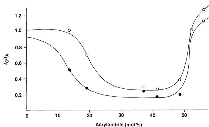
**Fig. 1.** Ratio of carbazole donor and anthracene acceptor emission intensities,  $I_C/I_A$ , in blends of equal weights of carbazole-labeled styrene-acrylonitrile copolymer and anthracene-labeled PMMA, as a function of the acrylonitrile (AN) content of the copolymer. The intrinsic viscosities of the PMMA in benzene at 25°C were 106 ml/g (○) and 18 ml/g (●). [Adapted from (14) with permission of the American Chemical Society, Washington, D.C.]
