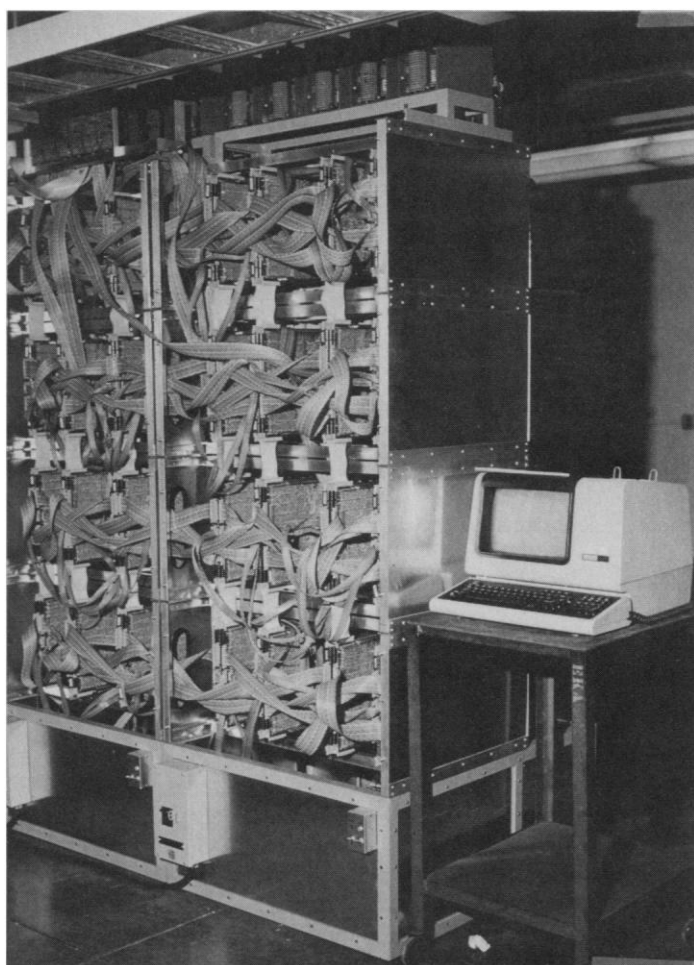
Fig. 5. Photograph of the 64-node Columbia machine. Each wire-wrap board is one of 64 identical processors. The wide ribbon cables provide data paths between neighboring nodes, while the narrow ribbon cables carry control signals between the nodes and the secondary controllers. This machine has the power of roughly six Cray-1 supercomputers and costs about $400,000.
