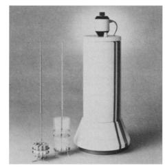
ing rates are proportional to the rotation speed of the fan. Specimens may be plunged into the liquid nitrogen without the chamber being opened. The 2195 holds ten 2-ml cryotubes or one hundred 0.25- or 0.5-ml straws. Nautilus Scientific. Circle 612.
