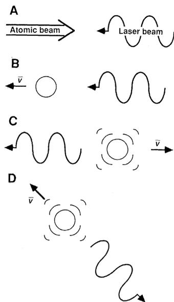
but low velocities are not attainable in this manner. A laser-cooled atomic beam, on the other hand, makes efficient use of the atoms, and achieves a narrow and selectable velocity. It has the additional advantage of being able to place all the atoms in a single internal quantum state and at quite low velocities.
