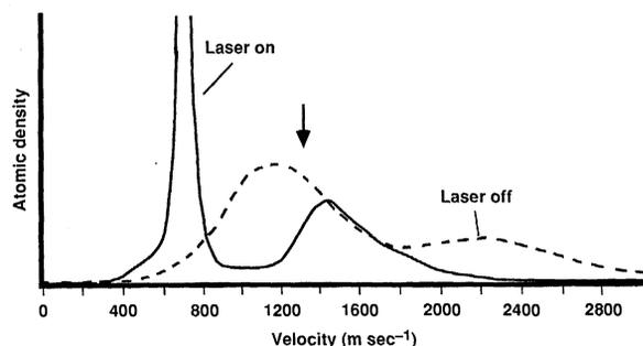
**Fig. 4.** Results of Zeeman-tuned cooling. Dotted and solid curves are as in Fig. 3. The arrow indicates the highest velocity resonant with the cooling laser. The velocity scale refers only to atoms in the  $F = 2$  state.
