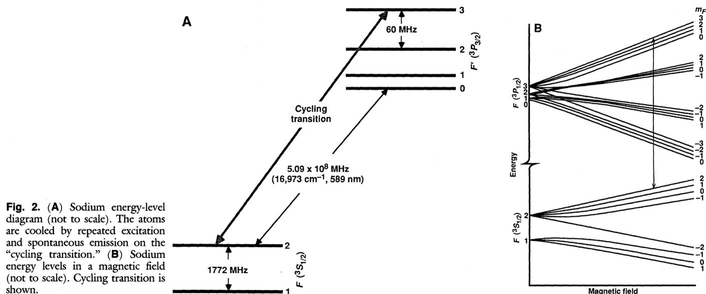
**Fig. 2.** (A) Sodium energy-level diagram (not to scale). The atoms are cooled by repeated excitation and spontaneous emission on the “cycling transition.” (B) Sodium energy levels in a magnetic field (not to scale). Cycling transition is shown.
