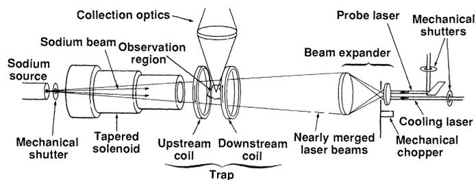
**Fig. 6.** Schematic of the apparatus used for the magnetic trapping of neutral atoms. The solenoid is 1.1 m long, and the trap is 40 cm from the end of the solenoid.
