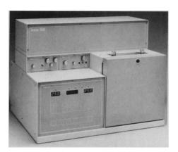
croprocessor-controlled model 540 also has five-level temperature programming, tenmethod storage, protected memory, and self-diagnostics. The large oven can hold megabore columns and features rapid heating and cooling. Tracor Instruments Austin. Circle 495.
