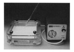
pump in 15 to 30 minutes. Molecules as small as 1 kilobase or as large as a chromosome may be transferred. Depurination, denaturation, and neutralization all occur within the VacuGene, and shakers, cassettes, wicks, and filter papers are not required. Reagents may be recycled. The VacuGene accepts gels as large as 18 by 23 cm. Pharmacia LKB Biotechnology. Circle 574.
