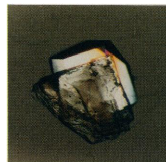
Fig. 3. Low-power microscope photograph (polarized light) of a crystal of lysozyme growing on a substrate crystal of the mineral apophyllite. The edges of the protein and mineral crystals appear to be parallel, which suggests possible alignment of the respective crystallographic axes.
