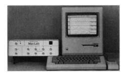
pare waveforms, and save data for later analysis. The hardware contains four differential high-gain input amplifiers, 12-bit analog-to-digital and digital-to-analog converters, and a microprocessor with 16 kilobytes of buffer memory. Two software packages are included; Scope emulates a single-channel oscilloscope, and Chart emulates a fourchannel paper chart recorder. MacLab operates with any Macintosh computer that has a free modem port. World Precision Instruments. Circle 569.
