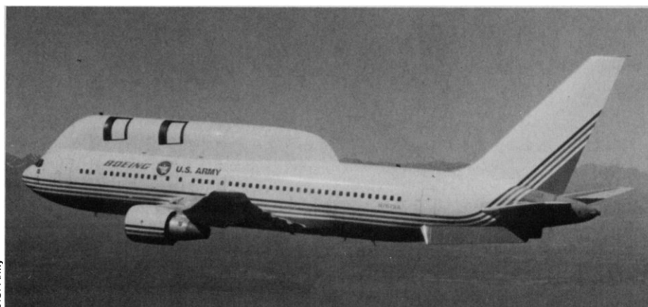
Airborne Optical Adjunct. An infrared sensor mounted in the aircraft will be used to track warheads in a controversial test.
