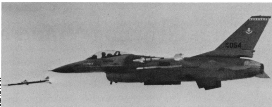
AMRAAM anti-aircraft missile , a new $500,000 item, uses radar guidance and may be vulnerable to radar-targeting or jamming.
