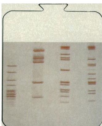
Analysis of DNA fragments from various digests by PAGE with subsequent silver staining detecting 75 pg. Range: 10 to 2000 bp. Sample to result: 70 min.
