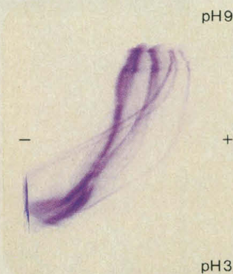
2-D titration curve on PhastGel IEF 3-9 with coomassie staining. Sample of beef muscle proteins. FROM SAMPLE TO RESULT: 60 MINUTES.
