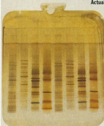
SDS-PAGE on PhastGel Gradient 10-15 with silver staining. Samples of meat and E. Coli proteins. FROM SAMPLE TO RESULT: 90 MINUTES.
