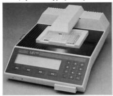
ware as well as configuration of the data transmission parameters and printer setup. Numbers and data are entered with a membrane keypad. Linear, semilogarithmic, and logarithmic-logarithmic regression analyses are possible. The MR 300 comes with a 410- and a 490-nm filter, and other filters between 400 and 650 nm are available. The MR 300 may be connected to a computer by means of an RS-232C cable. Dynatech Laboratories. Circle 552.
