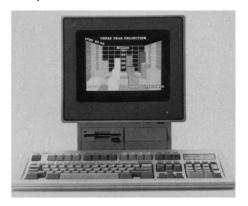
Multi Color Graphics Array (MCGA); the 12-inch monitor is available either in monochrome or color. Two expansion slots accept most IBM XT cards. The computer comes with either an 84-key or a 101-key keyboard. A collegiate version of the PS/2 25 is also available; it is configured with more memory, two disk drives, a mouse, DOS 3.3, and Microsoft Windows 1.04. IBM. Circle 531.
