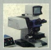
Discover the far reaches of inner space with the Polyspec microspectrophotometer. Able to scan the intermediate image in 0.05 micron steps, the Polsyspec can measure smaller features than any competitive microspectrophotometer. Yet, the compact Polyspec is so perfectly integrated that you can maintain all the functions your Polyvar delivers.
