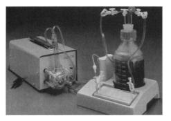
system's flat-plate design ensures even dispersion of cells and uniform nourishment by the media. Optimal levels of oxygen are maintained to encourage high cell densities. Cellular products are harvested separately from the cell bed. Millipore. Circle 631.
