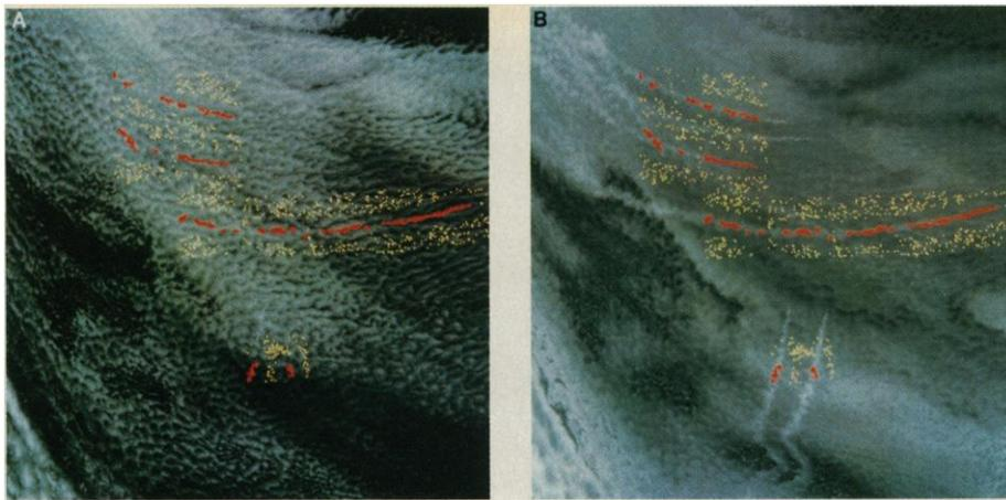
**Fig. 2.** Example of ship track identification (highlighted line segments) and randomly selected sample of noncontaminated clouds (bright dots): (A) superimposed on the image of 0.63- $\mu\text{m}$  reflectivity and (B) superimposed on the image of 3.7- $\mu\text{m}$  radiances.
