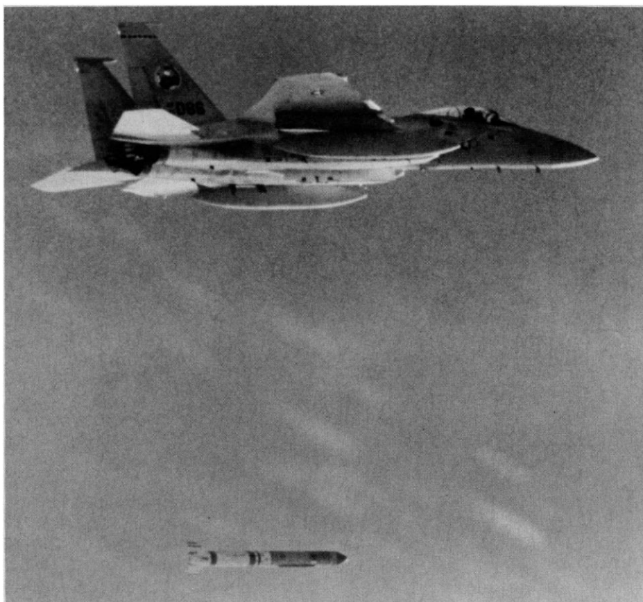
ASAT launch. The current U.S. ASAT consists of a miniature homing vehicle launched by a missile fired from an F-15 fighter.
