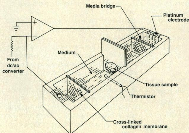
**Fig. 2.** Experimental apparatus for exposure of FPCM samples to electrical fields. Platinum electrodes were separated from the site of the tissue sample via media bridges. A programmable current source with series dc blocking capacitors maintained a constant current within the chamber media, independent of variations in electrode-electrolyte interfacial impedance. The lumen of the sample holder established a defined current density, and therefore field intensity, through the FPCM.
