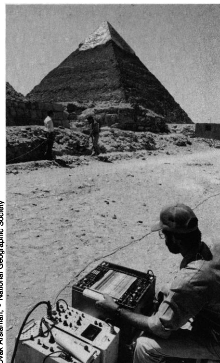
Radar profiling. Ground-penetrating radar is used to get a fix on the buried chamber, which is about 40 feet long, 8 feet wide, and 8 feet deep.
