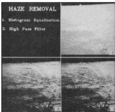
Histogram Equalization and High Pass Filtering for Reconnaissance Photos.
