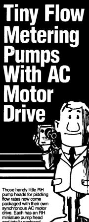
miniature pump head and totally enclosed three-speed motor drive assembly. This provides a choice of 150, 300 or 600 piston strokes per minute by means of a safe and simple belt change arrangement. Motor can be stalled indefinitely without overheating!
