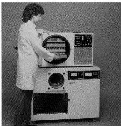
Dura-Dry™ condenser with Dura-Stop™ tray dryer—production-size performance in a laboratory-size tray dryer.
