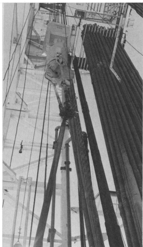
The needed power. This lifting block can handle 680,000 kilograms of drilling pipe, 2 kilometers of which is seen here stacked on the rig. This is part of the 1.6 million kilograms of equipment on the site that costs about $15,000 per day to operate, a good buy made possible by the depressed state of oil exploration.
