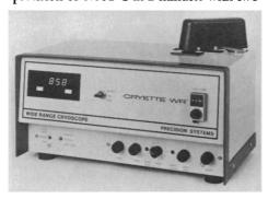
2.5-ml samples. The samples may be completely recovered after the freezing point is determined. The Cryette WR can also measure molecular weight of hydrocarbon fractions and determine solution concentrations. Precision Systems. Circle 546.
