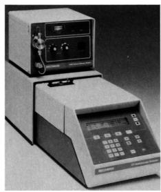
easy decontamination. Self-adjusting circuitry optimizes counting conditions for packed cells or liquid cells. Other features include a four-line, 40-character, liquid crystal display, menu-driven programming, automatic fraction-collector control, luminescence correction, automatic background subtract, automatic start and stop, and user-accessed diagnostics. Beckman Instruments, Nuclear Systems Operations. Circle 525.
