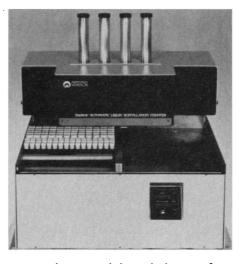
assays to be counted through the use of any of the 16 user-entered and user-selected protocols. The protocols—including the counting parameters of isotope count time, quench, and background counts—may be customized for each user. The TAURUS features preset isotope settings for <sup>3</sup>H, <sup>14</sup>C, and <sup>32</sup>P. Micromedic Systems. Circle 594.
