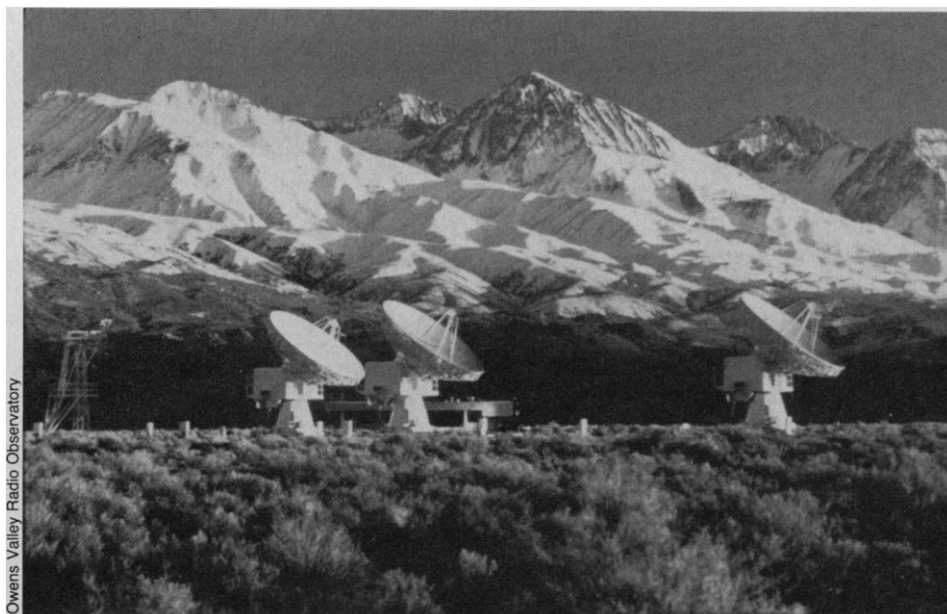
The Owens Valley millimeter-wave interferometer. Operated by the California Institute of Technology, the recently constructed interferometer consists of three movable radio telescopes, each 10.4 meters in diameter. At their widest separation they have the resolution of a single dish 100 meters across.
