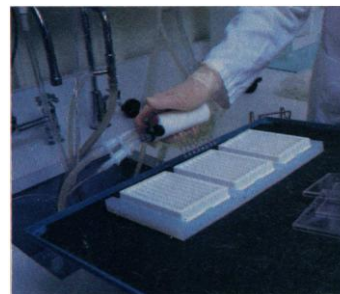
Immuno-strip washer—time-saving aspiration/delivery system.
