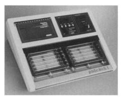
gel and optimizing the running buffer, the work station reduces the duration of electrophoresis to about 2 hours. In-cartridge conditioning and vacuum-assisted transfer moves the DNA from gel to membrane in two additional hours. Probe Tech 1 processes one or two gels of 11 lanes each. It is sensitive enough to detect DNA in fragments of 100 to 25,000 base pairs. Gels need only be handled twice—once when loading and once when removing them after transfer. Oncor. Circle 584.
