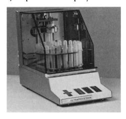
and sealed reagent vials. Specimens are moved from vial to vial without cross-contamination. The 3189 Ultraprocessor accommodates all specimens embedded in resin, whether destined for light or electron microscopy. RMC. Circle 550.
