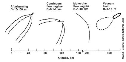
**Find the target.** As a rocket ascends, its plume changes dramatically, flattening out so that, by the time the rocket is above 200 km in altitude, the plume is as much as 10 km wide. The math problem is to find a way to locate the relatively tiny rocket in the plume.
