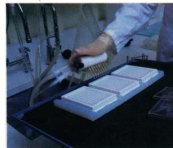
Immuno-strip washer—time-saving aspiration/delivery system.
