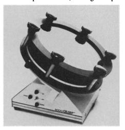
cially for users who require sterile conditions. The Celsep fractionates heterogeneous populations of cells into functionally distinct subpopulations. The Celsep system uses the principle of velocity sedimentation combined with chamber reorientiation to separate cells at unit gravity. Most heterogeneous cell suspensions, such as human leukocytes, bone marrow cells, and mouse spleen cells, can be separated with high reproducibility. Wescor. Circle 546.
