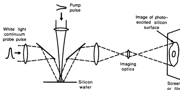
Fig. 5. Experimental arrangement used to obtain femtosecond time-resolved photographic images of a silicon surface undergoing an ultrafast phase transition.
