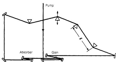
Fig. 1. The optical cavity configuration of a colliding-pulse, mode-locked dye laser with prisms inserted to compensate for the group velocity dispersion.
