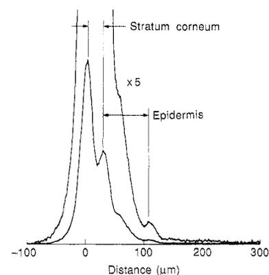
Fig. 9. Optical ranging measurement through human skin.
