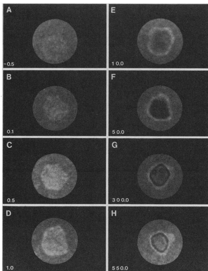
Fig. 4. Time-resolved photographs of a silicon  $\langle 111 \rangle$  surface after photoexcitation by an 80-fsec optical pulse. The numbers indicate the pump-probe optical delay in picoseconds. Note the rapid appearance of highly reflective molten silicon (B–D) followed by the ejection and dissipation of evaporated material (E–H).
